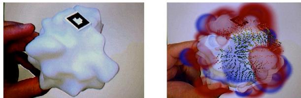
Figure 1: model of superoxide dismutase built with the Stratasys machine Prodigy Plus(left), overlay showing a volume render electrostatic field and animated electrostatic field vectors (right)
