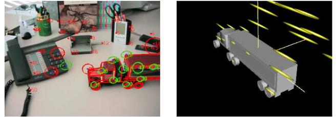
Figure 3: Uncertainties of the 3D feature locations projected into image space (left) and in 3D space from an external view (right).
