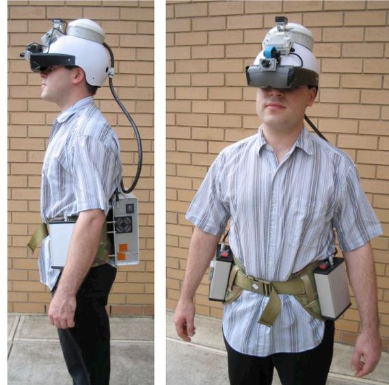
Figure 1 – The current Tinmith Backpack 2006 design presented in this demonstration. All components are fully contained within either the belt-mounted main case or the helmet, making the system small and robust.
