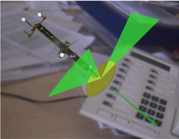
Figure 1: Mockup Visualization of predicted positional and rotational accuracy for a coordinate measurement tool
