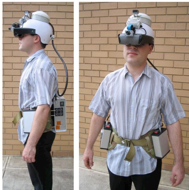
**Figure 1 – The current Tinmith Backpack 2006 design presented in this demonstration. All components are fully contained within either the belt-mounted main case or the helmet. Hot swappable batteries allow continuous operation.**
